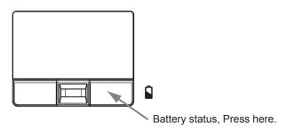
Once pressed, the 6 Status LED Lights will illuminate between 1 and 6 - The more lights illuminated, the higher the battery capacity of the battery, while the less lights, the lower the capacity.
